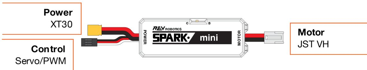
Connect the power wire to a free XT30 port on the REV Control Hub , REV Expansion Hub ([REV-31-1153](#)), or through an XT30 Power Distribution Block ([REV-31-1293](#)) that is connected to a free Control/Expansion Hub XT30 port. Connect the control wire to an open servo port on the hub and the motor wire to a JST-VH port on a motor, like the REV HD Hex Motor ([REV-41-1301](#)) or the REV Core Hex Motor ([REV-41-1300](#)).
