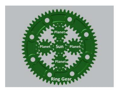
Interestingly, planetary gears can be used in a variety of ways with different gears serving as the inputs and outputs. For example, one might use the sun gear as the input and the planet carrier as the output while the ring gear is held stationary, or one might use the ring gear as the input and the sun gear as the output while the planet carrier is held stationary. The overall mechanical advantage of a planetary gear set changes depending on the configuration used.
