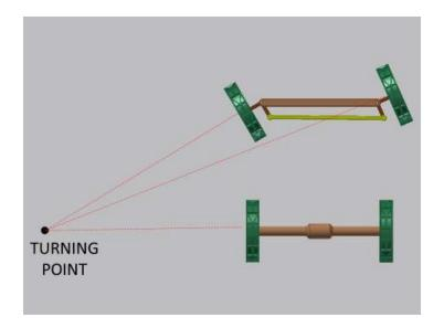
In this type of drive, all the wheels move in the same direction: forward or backwards. Steering is accomplished by turning the wheels such that all the wheels are positioned in an arc around a single turning point.
