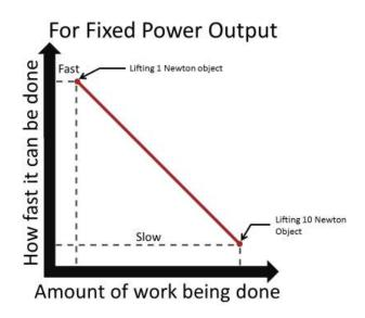
Power is defined as Force multiplied by Velocity (how fast one can push with a constant force), and is frequently expressed in units of Watts.
