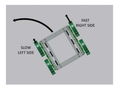
This type of drivetrain is capable of zero radius turns; the robot driver would simply power one side forward and the other side in reverse.
