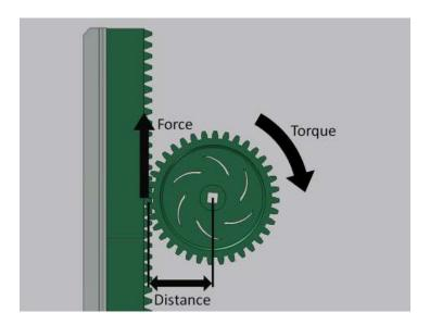
In the above example a <u>rack and pinion</u> mechanism is used to drive the elevator. The pinion gear spins at some speed with an applied torque. This torque then applies a linear force at the gear's pitch circle, which drives the mechanism.
