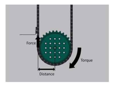
The above image shows how chain and sprockets can be used to drive a linear elevator. The torque on the driving sprocket spins the chain. The chain is attached to the linear elevator, and exerts a linear force to drive the mechanism.
