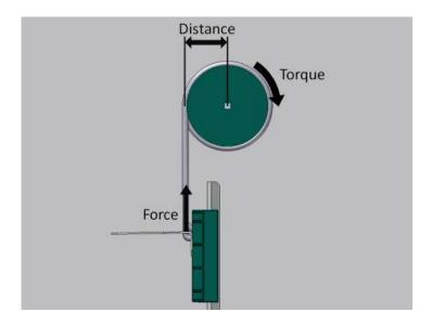
In the above example, a winch is used to drive a linear elevator. A motor applies torque to the winch which provides a linear force along a rope, which then drives the mechanism.
