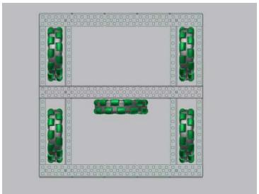
Since omni-wheels don't have any sideways friction, the wheels facing forward/backward can drive without the wheels facing right/left dragging. By powering both sets of wheels, the robot can move in any direction.
