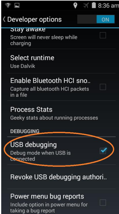
Figure 64 - Make sure USB debugging is enabled for your phone.
