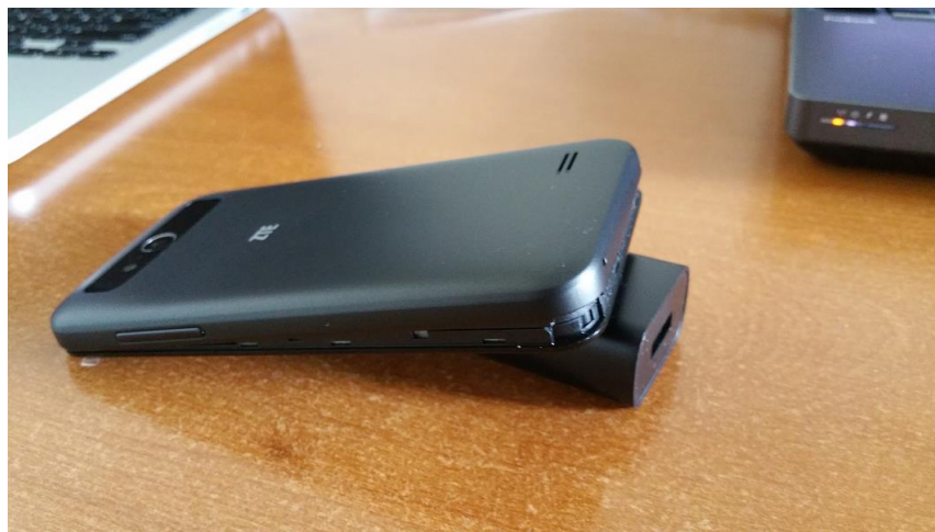
Figure 46 - Pry the back cover off of the phone.
