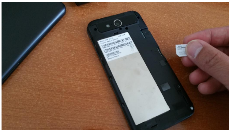
Figure 49 - Remove the card from its slot and replace the back cover.
