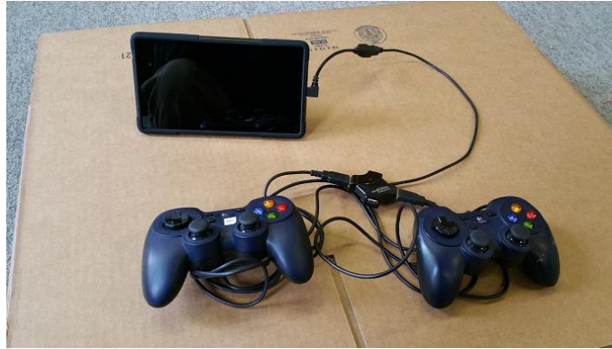
Figure 4 - Driver station hardware consists of a tablet, an adapter cable, a USB hub and two gamepads.
