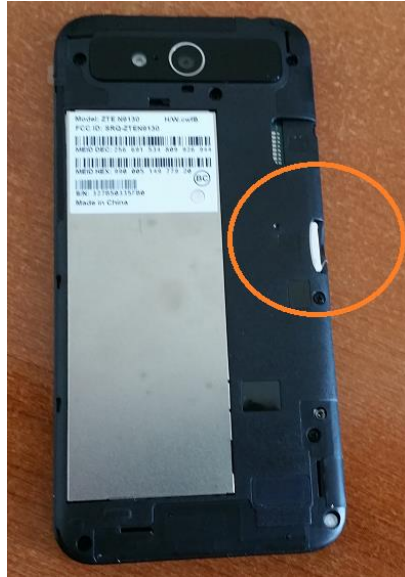
Figure 47 - The SIM card is installed in the right hand side.
