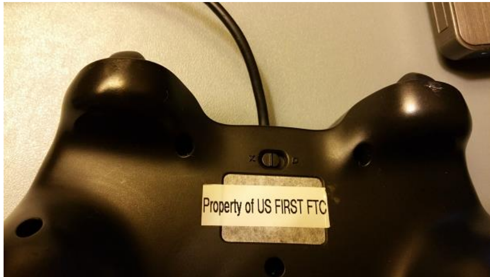
Figure 91 - Make sure the switch is in the "X" position.
