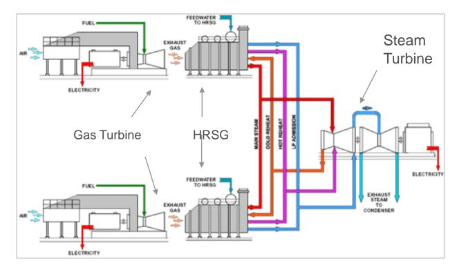
There are many possible configurations for Gas turbines and HRSG's. The drawing above shows the "2 on 1 "configuration found at many Southern Company Combined Cycle installations
