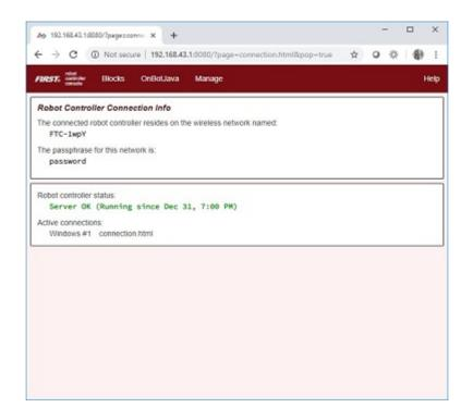
• Click on the Manage link towards the top of the Robot Controller Connection Info page to navigate to the Manage page.
